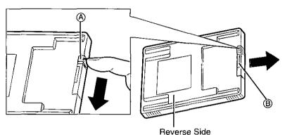
2 Install the battery with the plus side up, then insert the tray until it locks.
